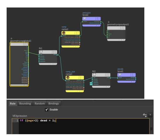
In the popvop node, I used ramp to control the pscale and color attribute on the points. To control the movements of particles, popwind and popdrag are good options for this project. Popkill node is used for controling the amount of particles which related to age attribute.
